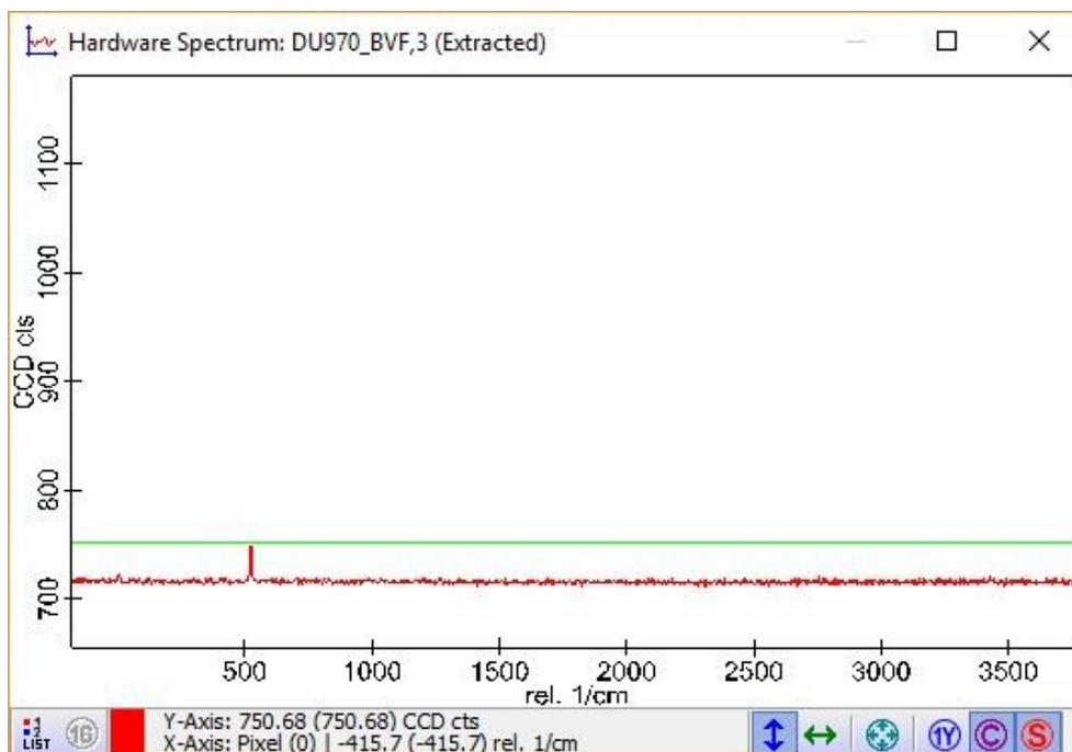
Figure 1: Low intensity silicon spectrum
