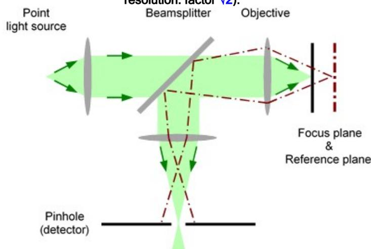
Fig. 1: Principal setup of a confocal microscope
