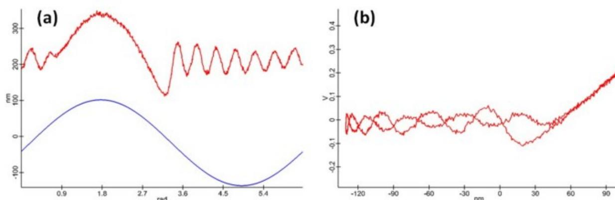
Fig. 9: Example of DPFM and  $f_{\text{modulation-distance}}$  curve displayed in one graph viewer (a) and force-distance curve obtained from a DPFM measurement (b).
