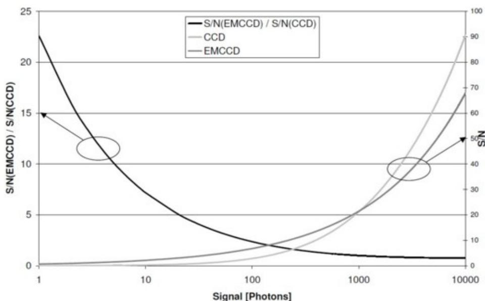
**Figure 1: The theoretical S/N for a "normal" CCD camera and an EMCCD camera as a function of the signal reaching the detector. The ratio of the two S/N ratios is shown as well.**
