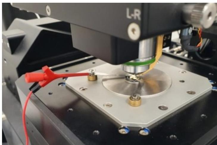
**Figure 2: Reference sample mounted on the microscope**
