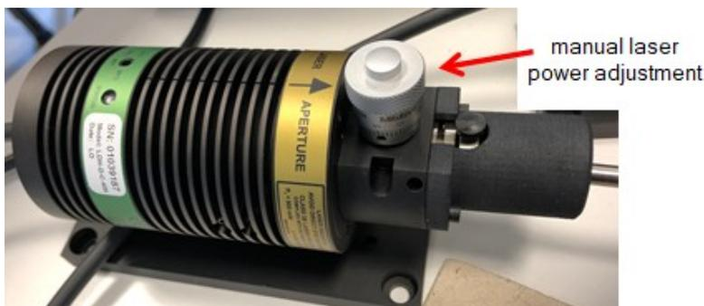
**Figure 2: PicoQuant LDH series laser head**
