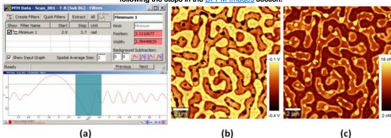
**Fig. 4: Evaluation of adhesion from the PFM curves using the filter manager of WITecProject in conjunction with the Minimum filter and the appropriate filter selection range (a), extracted image from the filter manager (b) and the evaluated adhesion image (c).**
