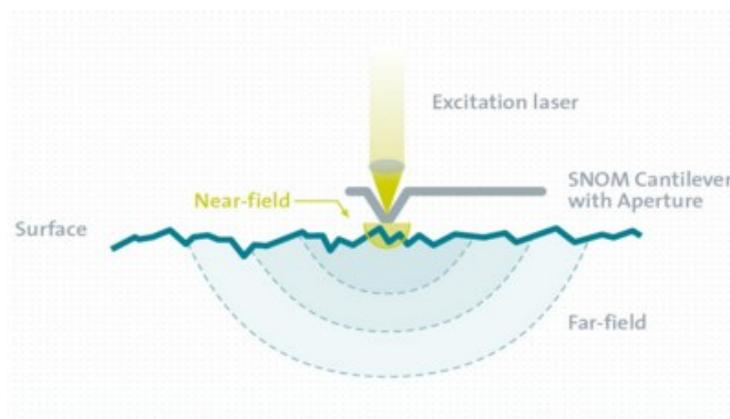
Scanning Near-field Optical Microscopy (SNOM) is a technique to achieve lateral resolution below the diffraction limit using an aperture and a point detector.
