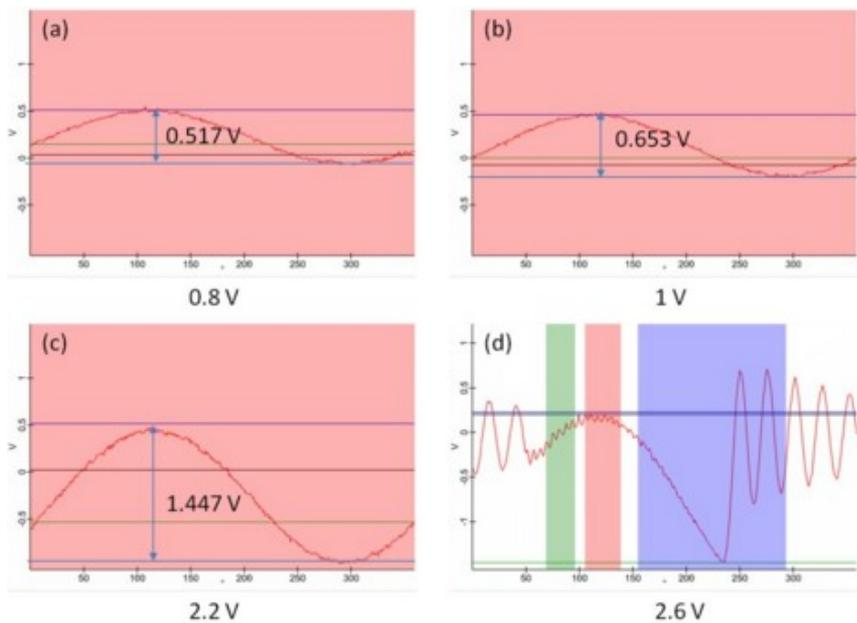
**Fig. 2:** Illustration of the oscilloscope window while measuring the modulation factor on a Si wafer at various driving amplitudes of (a) 0.8 V, (b) 1 V, (c) 2.2 V and (d) 2.6 V (where the cantilever is already detaching from the sample).
