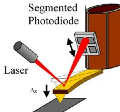
**Fig. 1: Principle of AFM operation.**
