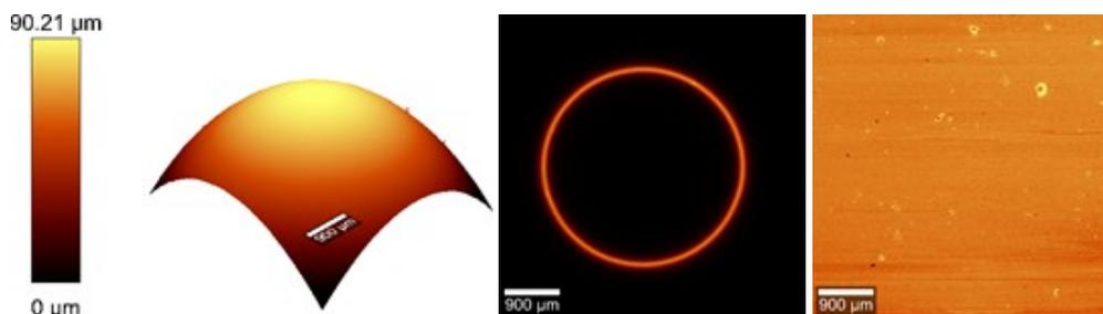
**Figure 1: Si lens. Left: Topography. Middle: Only one depth level is in focus with the standard confocal Raman microscope. Right: The same image as in the middle, but with TrueSurface activated the Si signal is constant from all depths as the sample surface is always kept in focus.**
