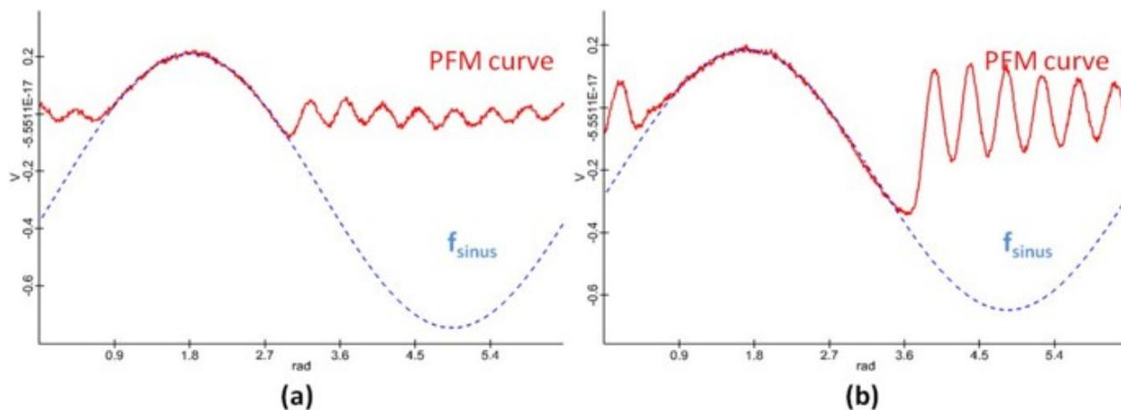
Fig. 8: PFM and  $f_{\text{sinus}}$  curves from a stiff (a) and soft (b) measuring point represented with the same y-axis.
