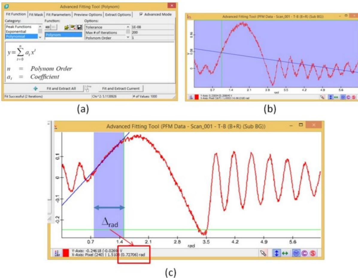
Fig. 5: Advanced fitting tool for 1<sup>st</sup> order polynomial fit (a), graph viewer which opens together with the fitting tool (b) and graph window showing the selected range of interest together with the blue fitting curve (c).
