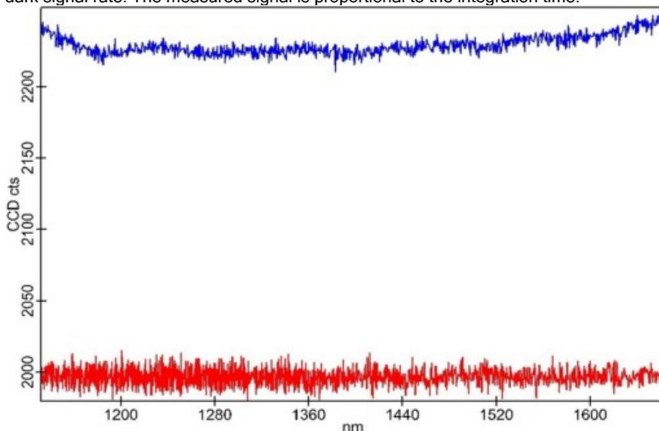
Fig. 4: Single spectra without (blue) and with (red) dark current correction (0.5 s integration time).
