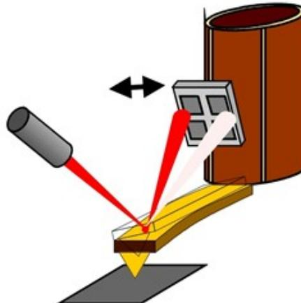
**Fig. 3: Principle of AFM friction measurements.**
