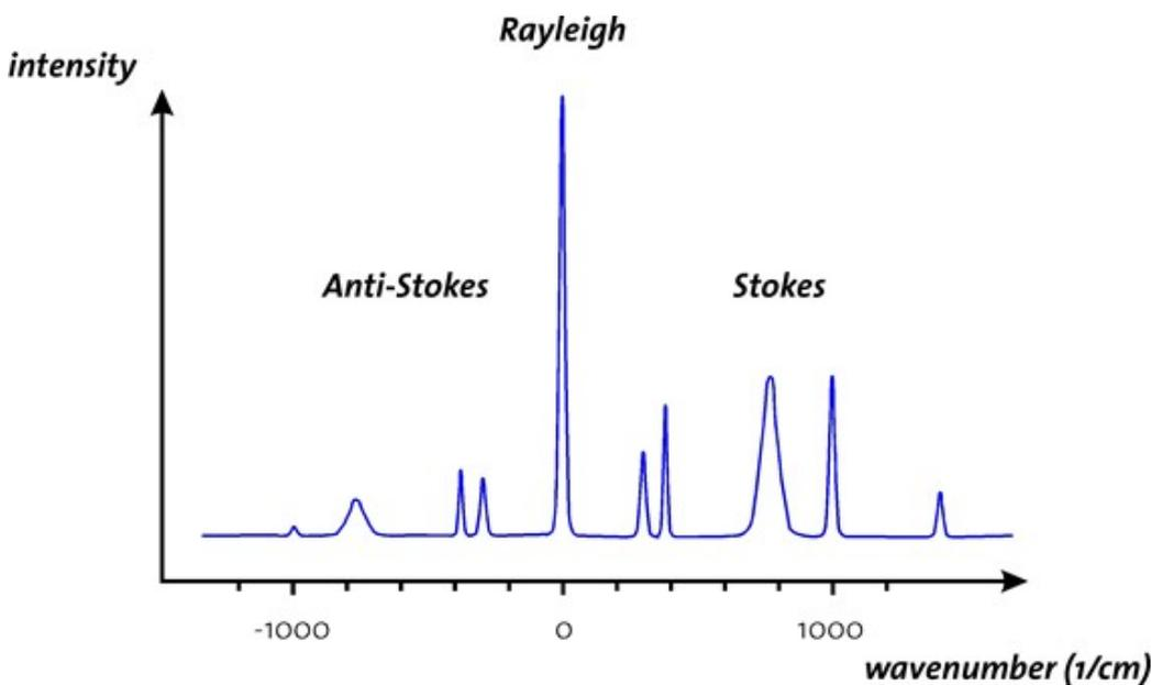
**Fig. 2: Typical Raman spectrum**
