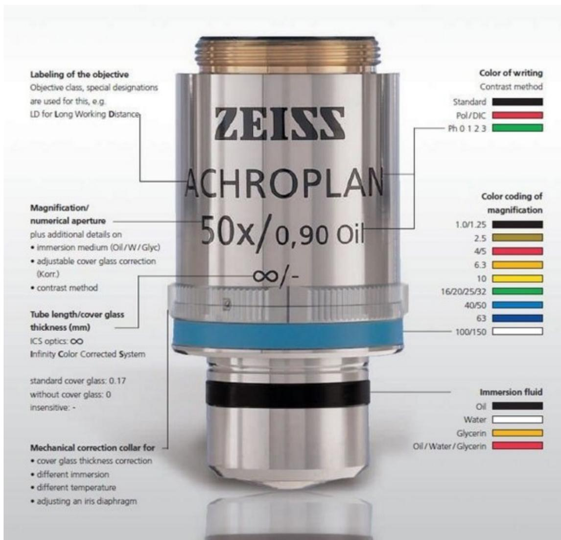
Figure 1: Labeling of Zeiss objectives (Source: <https://www.zeiss.com/microscopy/int/products/microscope-components/objectives.html>)
