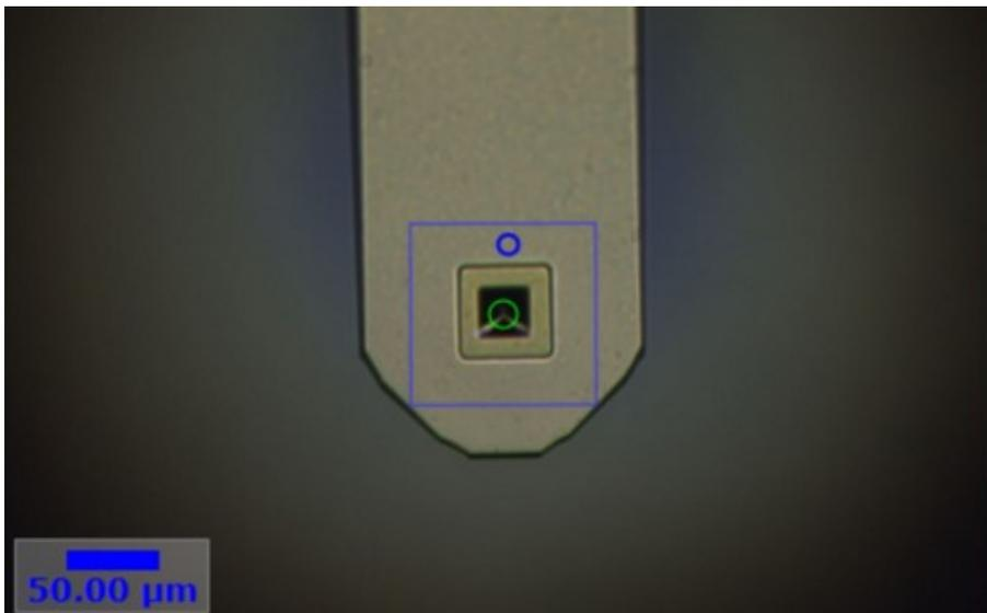
Fig. 1: SNOM cantilever focused into the aperture (top view)
