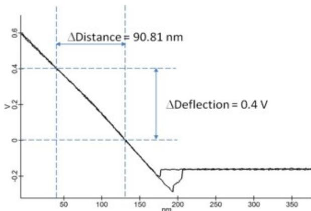
**Fig. 1: Force-distance curve measured in contact mode on a Si wafer.**
