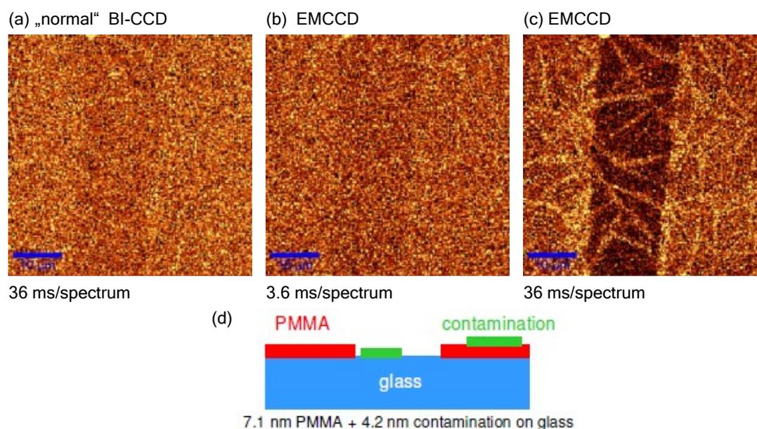
**Figure 2: Confocal Raman Images of a 7.1 nm PMMA layer on glass obtained in the CH<sub>2</sub> stretching band around 2950 cm<sup>-1</sup>: (a) back-illuminated CCD, (b,c) EMCCD. Scale bar: 10μm. (d) Schematic of the sample.**
