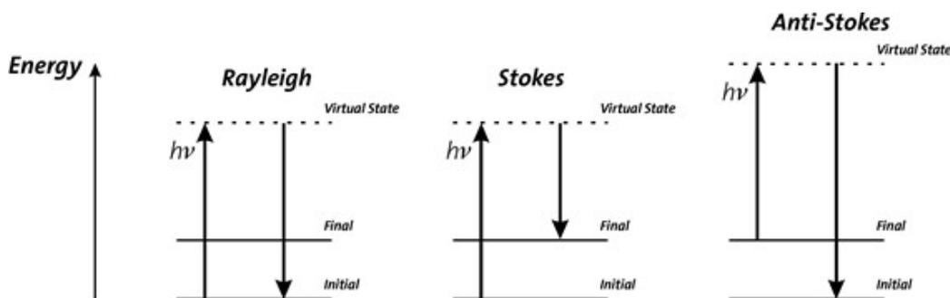
**Fig. 1: Energy level diagram for Raman scattering**
