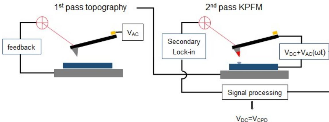
**Figure 1: KPFM measurement principle**
