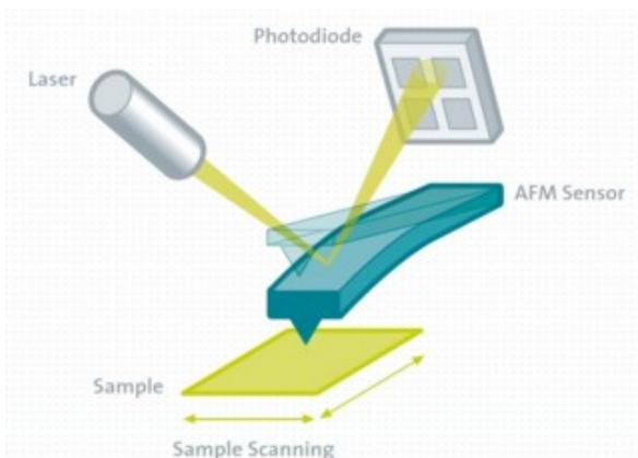
Atomic force microscopy (AFM) is a type of scanning probe microscopy (SPM), where the sample is scanned mechanically on the nanometer scale. Besides the sample topography additional properties can be determined with special AFM modes.
