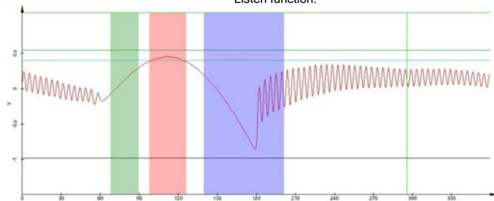
Fig. 2: Pulsed force curve with Fmax (red), Adhesion (blue) and Stiffness (green) search window
