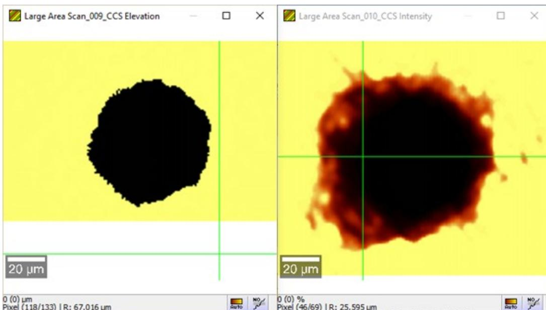
Figure 2: Pinhole with CCS sensor
