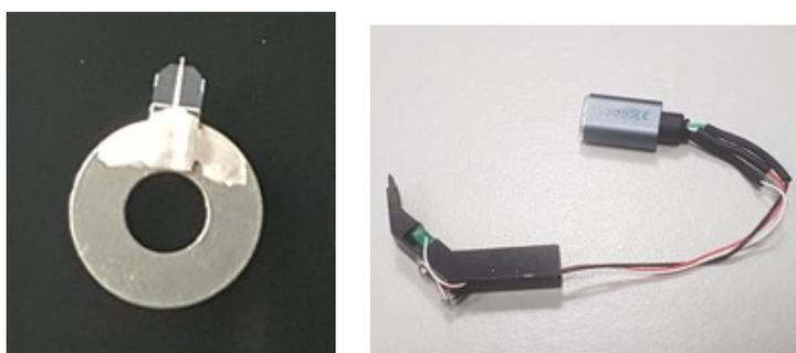
Figure 1: Cantilever connected with silver conductive paint (left) and EFM arm with electric connection (right)
