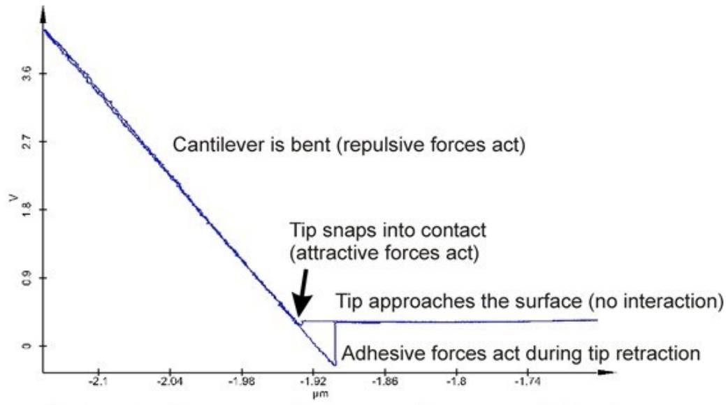
**Fig. 2: Force distance curve in an AFM measurement.**
