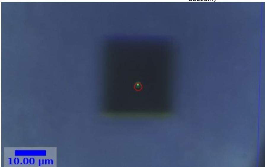
Fig. 2: SNOM cantilever with transmitted light (bottom view)
