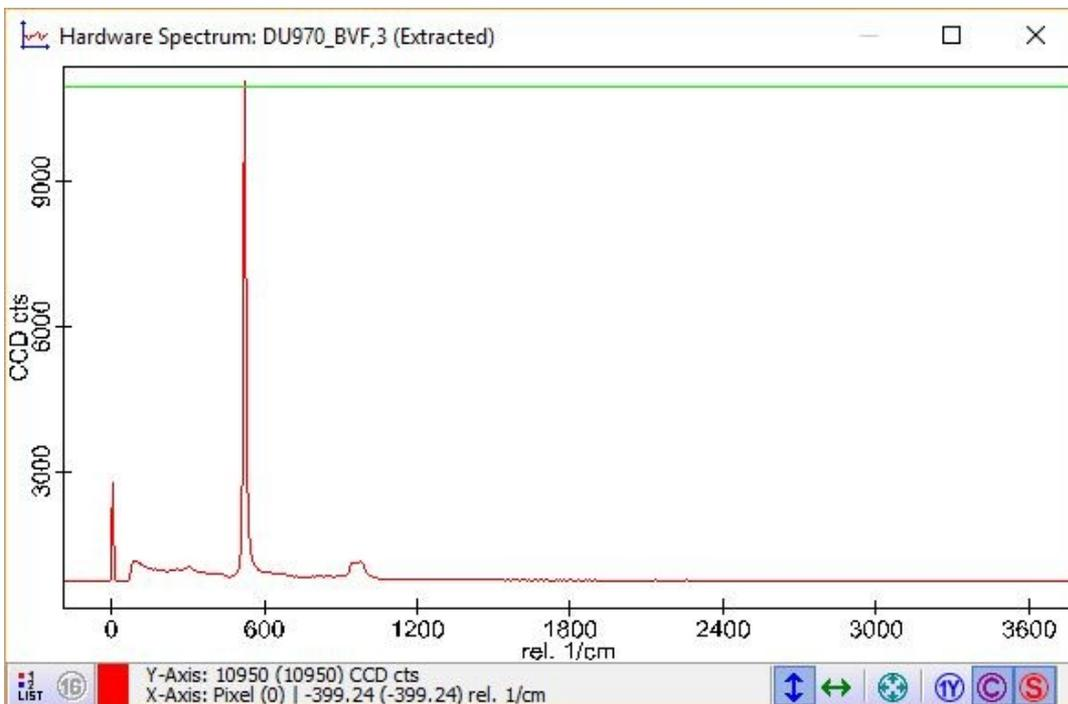
Figure 3: Silicon spectrum with optimized fiber position
