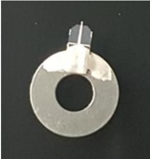
Figure 1: Cantilever connected with silver paint
