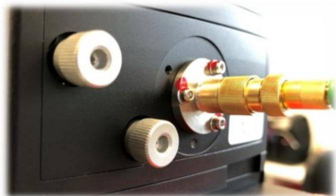
Figure 2: Fiber alignment screws
