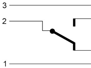
Relay switched on: contact between pin 2 and pin 3 (Meaning an emergency program has been triggered.)
