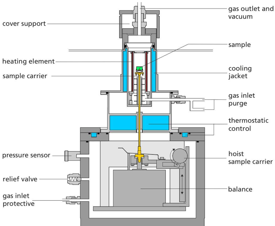
Figure 2: TG 209 F1 measuring cell (schematic)
