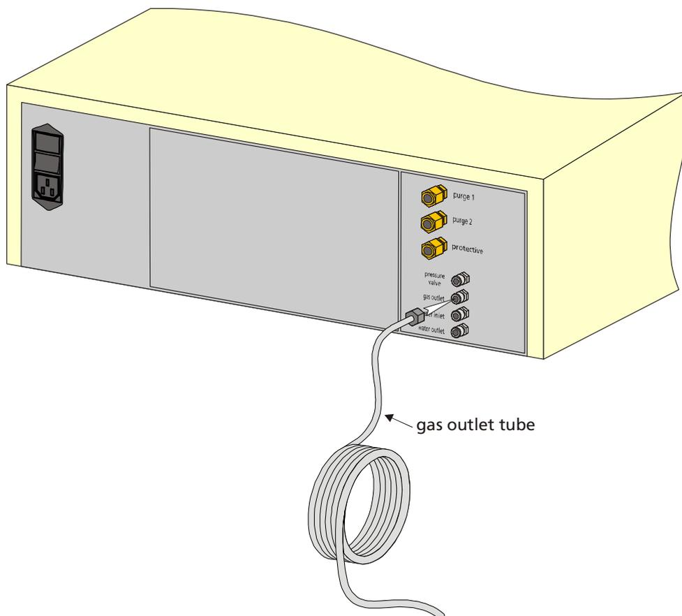
**Figure 8: Connecting gas outlet tube**
