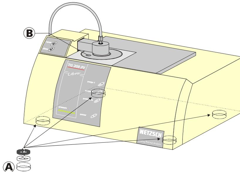
Figure 2: Alignment measuring unit
