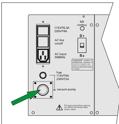
Figure 6: Electrical connection of the evacuating system
