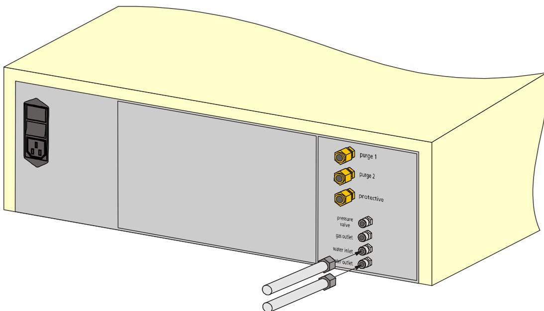
Figure 4: Connecting thermostat
