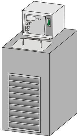
A thermostat is required to operate the instrument. This handles thermostatic control of instrument components relevant to the measurement and cooling of the furnace system. The thermostat is connected to the **thermostat (inlet-outlet)** connections on the back panel of the measuring unit.
