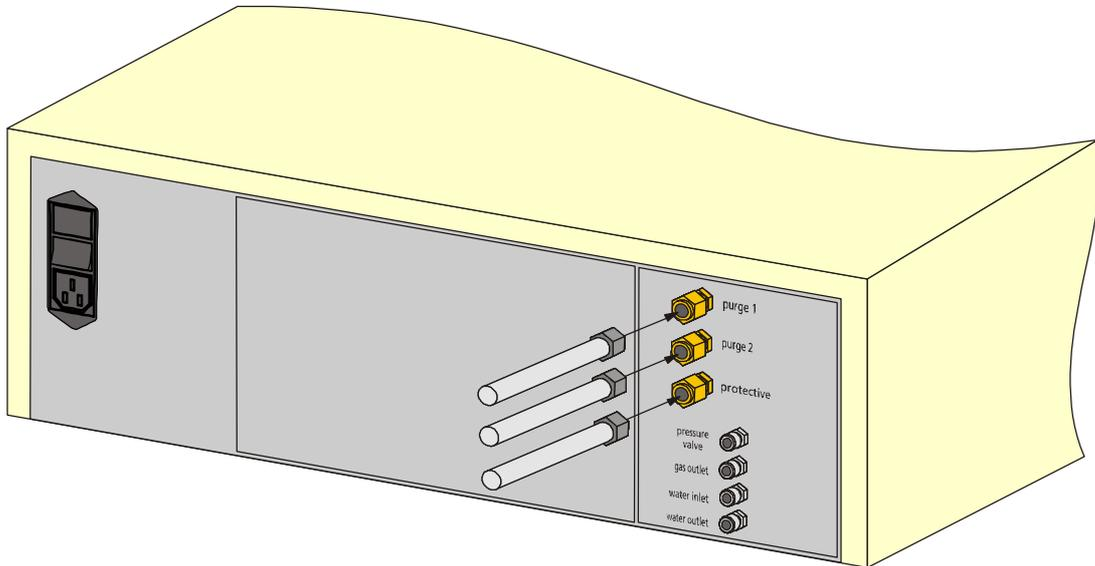
Figure 7: Connecting gas supply
