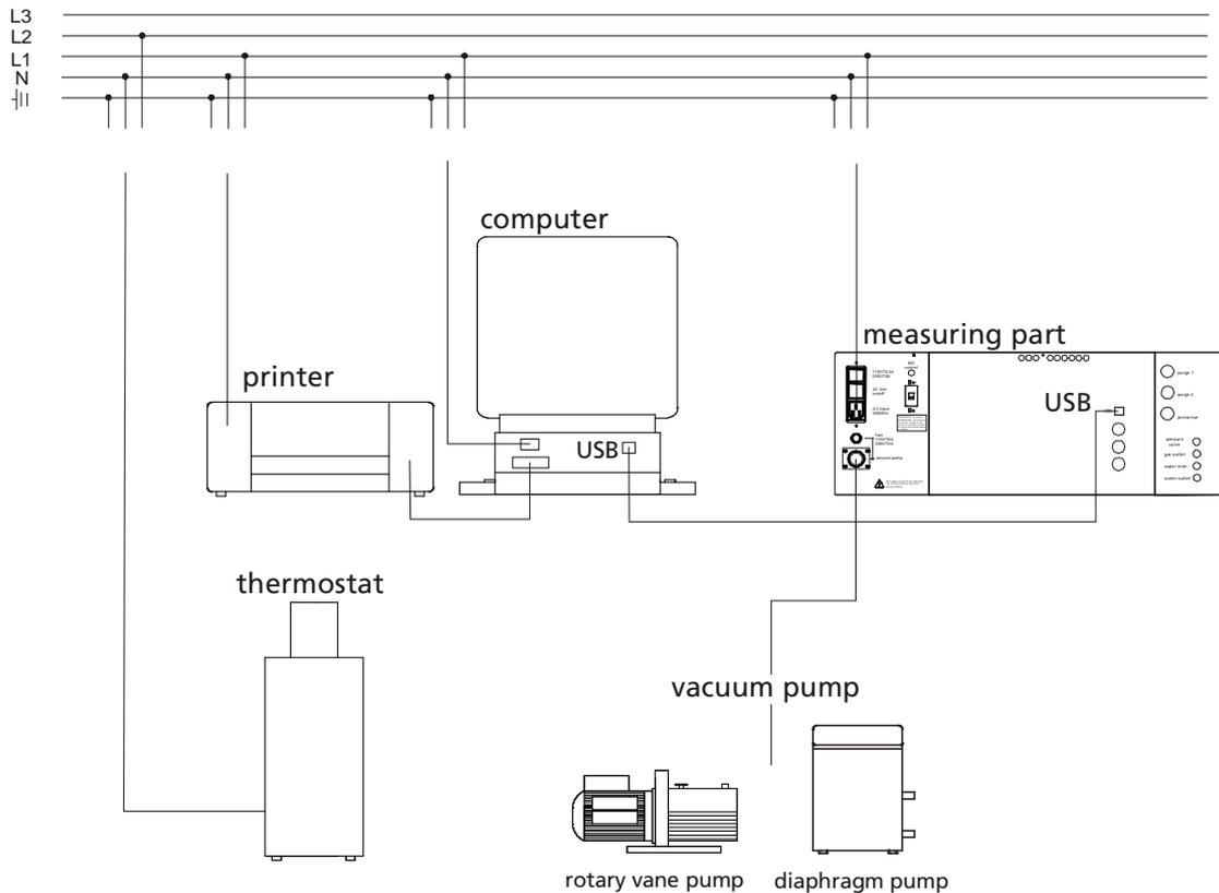
Figure 3: Electrical connections
