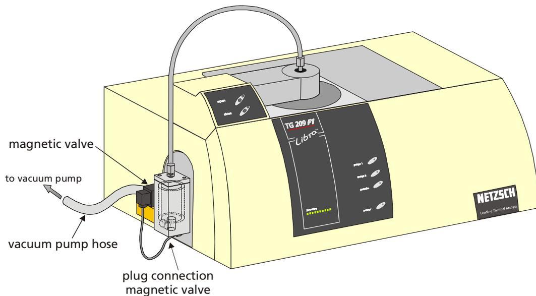
Figure 5: Connecting the evacuating system
