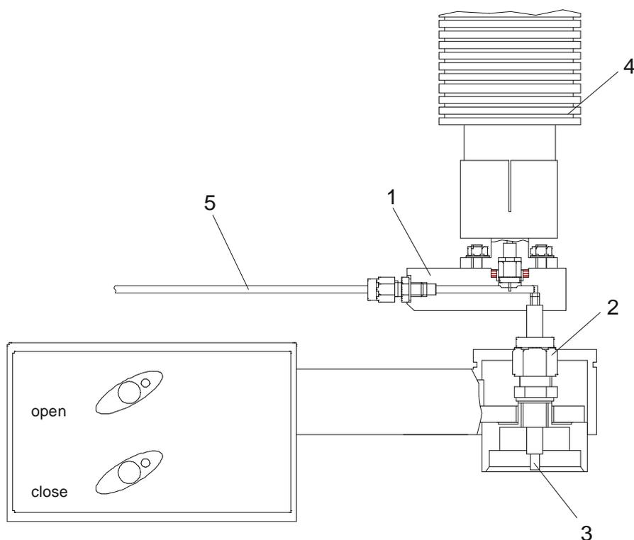
The adapter head (1) is attached by the screwing (2) on the cover of the TG 209 F1. The gas tube (3) can be unscrewed for cleaning. The transfer line (4) is fixed upright to the gas flow on the adapter head. The excess gas is dissipated via the gas outlet (5). The adapter can be heated up to 300°C.
