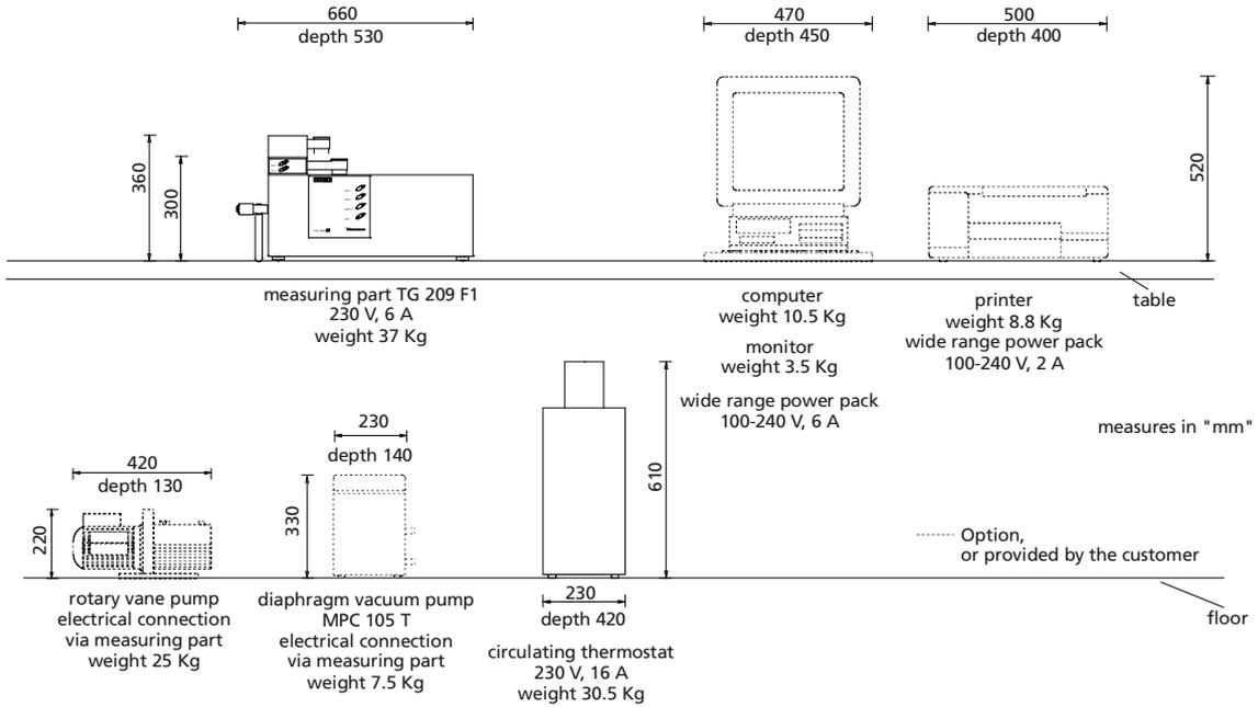
Figure 1: Installation schematic TG 209 F1
